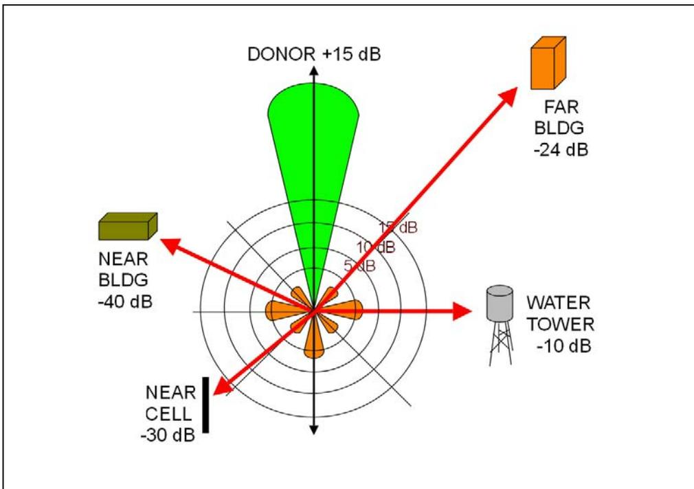
This illustration shows the practice of slightly rotating a directional antenna 'off center' so that the offending sources fall with the low gain side lobes of the antenna. This effect is most noticeable in Yagi type antennas.
