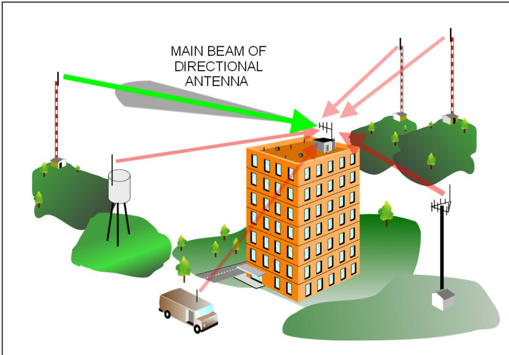
The above illustration shows the importance of a directional antenna in reducing the levels of potential undesirable interferers. Note the vehicular source also.
