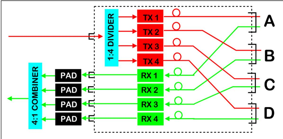
Note that each FO receiver output at the repeater site has individual pads to reduce the composite noise floor and provide FO RX to FO RX isolation and minimize receive combiner intermodulation. For example, if 40 dB pads are used, an additional 80 dB of combiner port-to-port isolation occurs.
