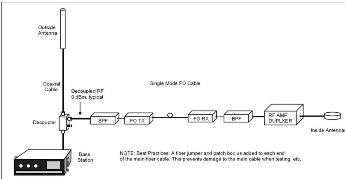
The RF source is a decoupled signal from a RF transmitter (Base Station or signal booster). The full output power of the RF transmitter would damage the FO TX. Assuming the RF transmitter is also connected to an outside antenna, the decoupler used is a directional type to further reduce any unwanted signals that
