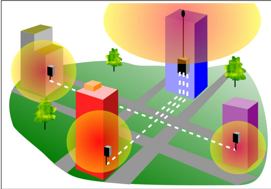
Unused single mode fiber optic cables often already connect the buildings for data communications and spare fibers can be used for the RF over fiber system to enhance radio signals in the other buildings.
