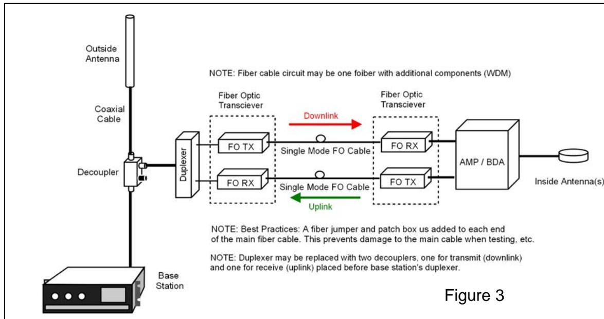
The fiber equipment located at the base station (or signal booster) is the head-end. The equipment located at the other end of the fiber cable is the remote -end.
