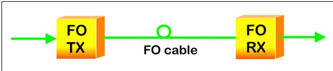
In this example, RF from a RF transmitter is injected into the FO TX (Fiber Optic Transmitter) at one end of the fiber optic cable. At the other end of the cable, the Fiber Optic Receiver (FO RX) converts the signal back to RF. The input level is 0 dBm typically and the output level is equal to the input level. Note there is a net zero loss of RF signal end-to-end.
